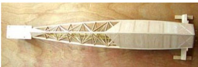
The first picture below shows the 1/16" stab mounting platform now glued on to the fuselage longerons. The top longeron had to be removed in order to mount the stab platform. The two plywood inserts integrated into the platform where the nylon mounting screw holes are.
