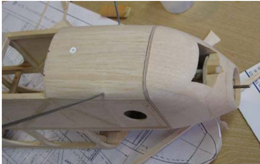
This last picture shows how the clean lines of the cowl streamlines the front of the fuselage and mates with the spinner.
