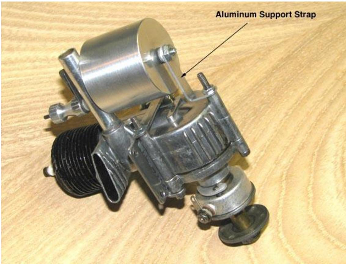
**TANDY WALKER**, our member in Arlington Texas produces some really sanitary looking models and engines. Here's a neat tank support strap he made to add stability to an aftermarket metal tank so he could run methanol in his O&R 23. Those hanging tanks on O&R's are a nuisance as they often wiggle around and come loose. Tandy says he got the idea from Vic Didelot before he passed away. We haven't run an O&R tuning tip in the series for a long time, so we'll call this one **O&R Tuning Tip #22**.
