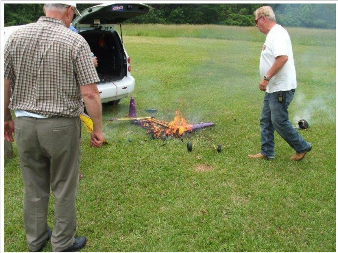
**LITHIUM BATTERY FIRE!** Mike Keville, former OT Columnist for Model Aviation sent this picture of the fire that can happen when you charge Lithium batteries and the charging procedure goes awry. Sometimes there's an explosion along with the fire. There's not much of anything useable left which is why they recommend charging these batteries outside the aircraft. Let's hope the ship wasn't in the car trunk at the start.
