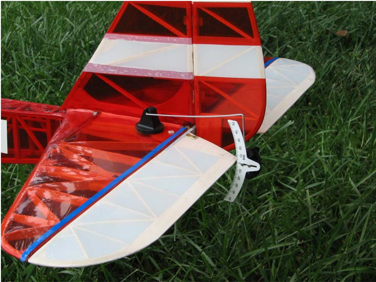
Here's the Great Planes deflection gauge in use. That spring arm and black pad on top has a twin on the bottom. This allows you to quickly clip it onto a control surface for measurement.
