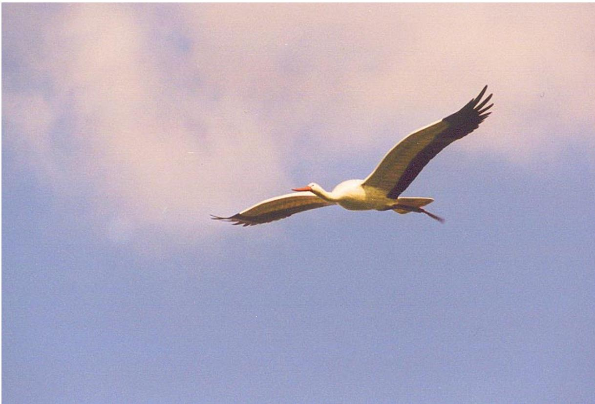
Believe it or not you're looking at an electric RC model of a stork. It was built in Germany using a complex geodesic internal framework. The motor is up front and a long drive shaft extends to the rear propeller. That prop folds back during glide to become the storks' legs which normally trail behind in flight just as you see in the picture.
