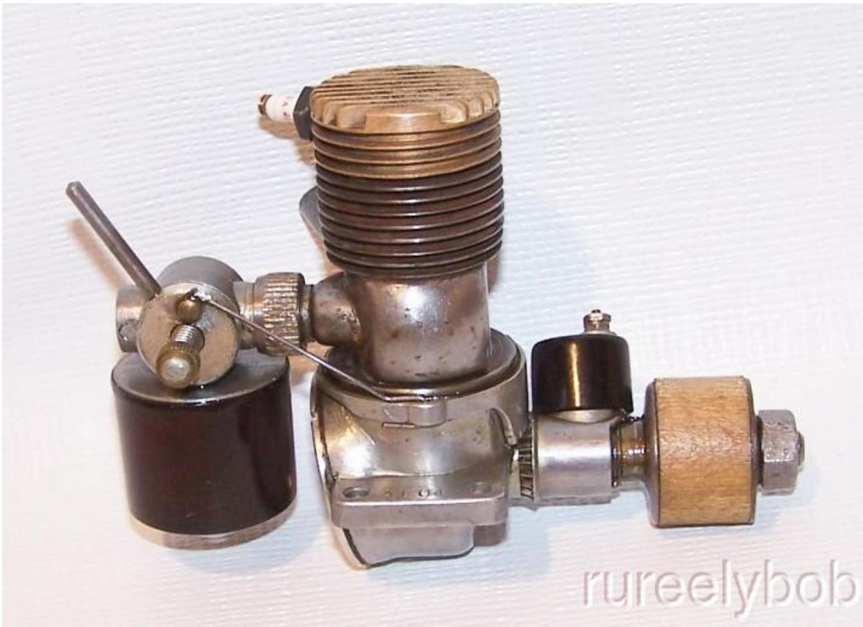
And here we have a Condor Copper King. It's maybe a little less rare than the Bond above. It looks to have a similar adjustable enclosed fixed point. Notice how the throttle lever advances the timer through a linkage and gear arrangement.
