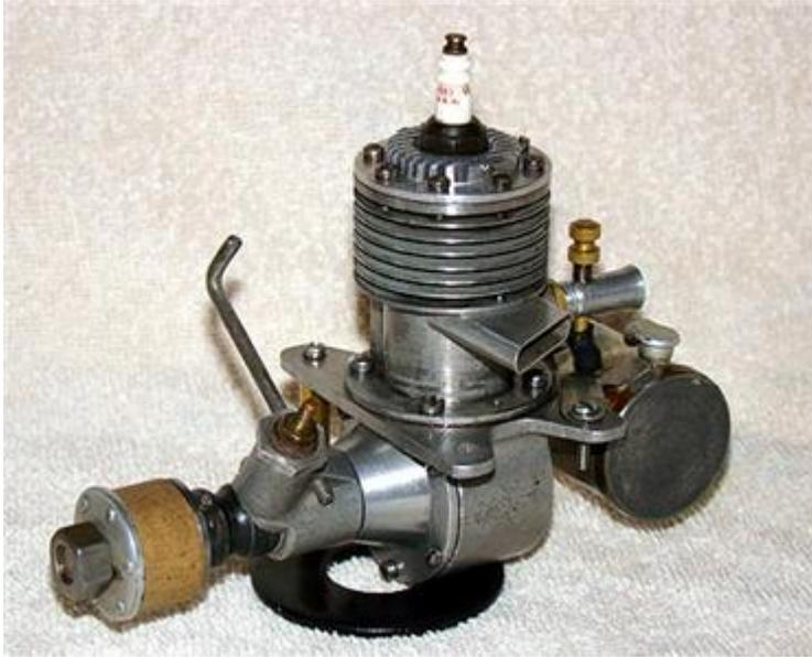
Here are a couple more engines you will probably never see on the flying field. This one is a Bond BRL "A" model. I believe it had .56 C.I. displacement. Notice the apparently simple adjustment on the enclosed fixed point.
