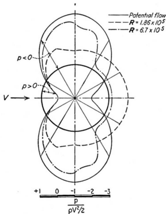
FIG. 100.—Pressure distribution around a circular cylinder.
