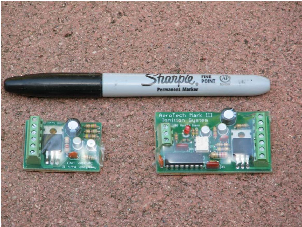
**THE MK II AND MK III** ignition units above are new offerings from Marvin Stern. The MK II at the left performs functions similar to Larry Davidsons “SSIGNCO” solid state spark trigger which we tested and reported in our Feb. 2010 issue #244. The units may have been developed in response to a need pointed out in the Old Timers column in Model Aviation.
