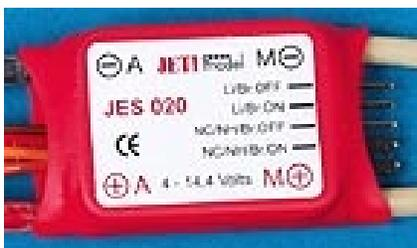
This is an ESC or Electronic Speed Control in approximately its' actual size. approximately its' actual size.
