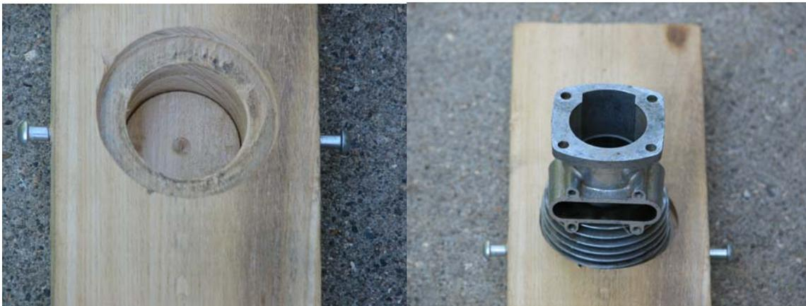
Here's the inertia puller: The hardwood board is about 2 feet long. Forstner bits were used to drill the two concentric flat bottomed holes. At the right we have the cylinder in place before it's strapped down with rubber bands.
