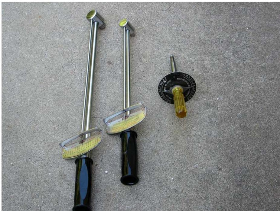
The large wrench is calibrated in foot pounds and for you metric enthusiasts it has a second scale in meter kilograms. At its' max reading, 140 ft. lbs. = 19.36 meter kilograms.
