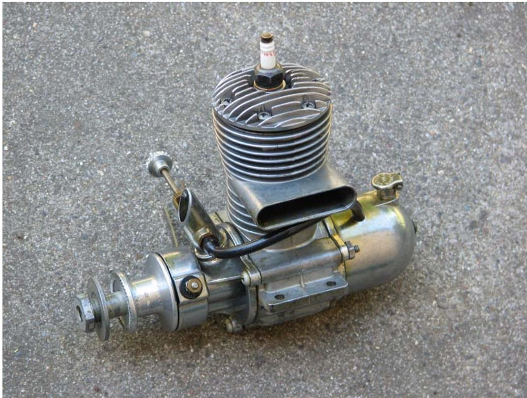
This good looking and nicely built engine came in both .49 and .51 displacements. The one pictured happens to be a .51. The only external difference is a 49 or 51 stamped on the top of a mounting lug. Like other engines of the postwar era, they were soon furnished as glow models. Those remaining today seem to be about evenly divided about between glow and ignition models, and also between the two sizes.
