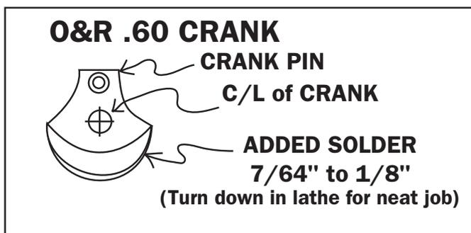
Have you looked at a new O.S. or Enya engine? Even though the piston is light aluminum or iron in the small sizes, the crank counterweight is quite large. We are told that a single cycle engine cannot be truly balanced, but a formula exists that comes as close as possible to the physics involved. Take 1/8 the weight of the rod and 1/4 the weight of the piston and put it on the crank counterweight. This states it in general terms.
