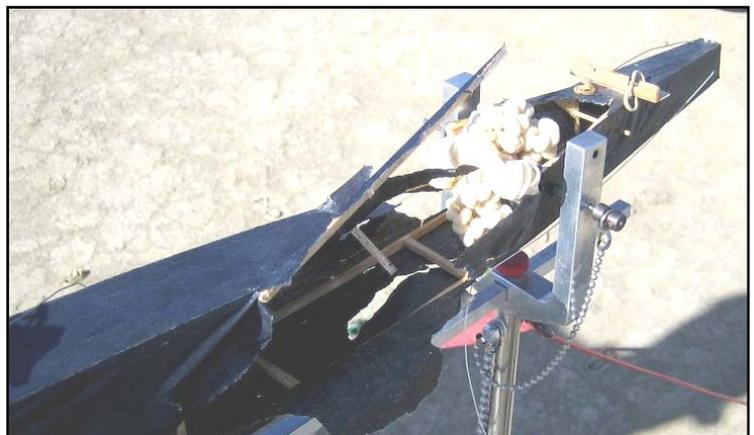
The motor let go as Bernie was inserting the propeller on this Joe Williams Moffett after winding and after removing the blast tube
