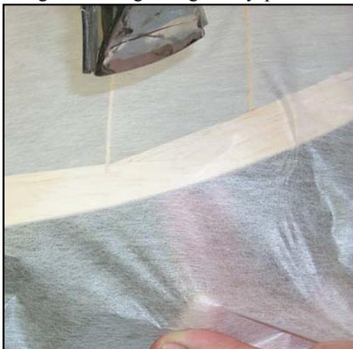
Shrinking out the extra covering formed when going around a compound curve tip. This is a 1/2 Texaco Powerhouse tip covered with regular Polyspan (note next wrinkle to shrink on right side of picture)
