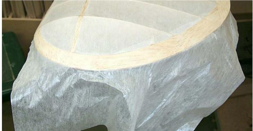
Same tip on 1/2 A Texaco Powerhouse after all the wrinkles were shrunk out and stuck down. Works great and no need for a splice to get around the tip!
