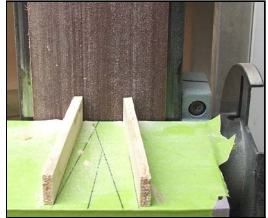
Sander set with guides at 11 degree angle
