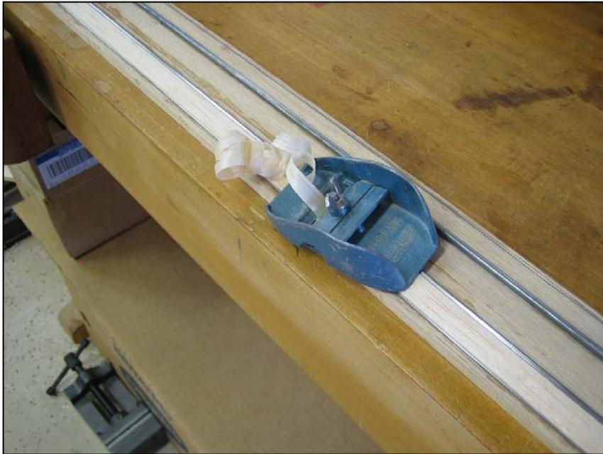
The rectangular stock is pressed into place between the wires with the far end resting against the stop. It is then stripped down with a hand razor plane using the piano wires as guides to set the angle and get the required thickness (Fig 4.) Once the work piece is close to the desired thickness, it can be finished off with a sanding block of suitable grade paper. The attached pictures make all of this pretty clear.
