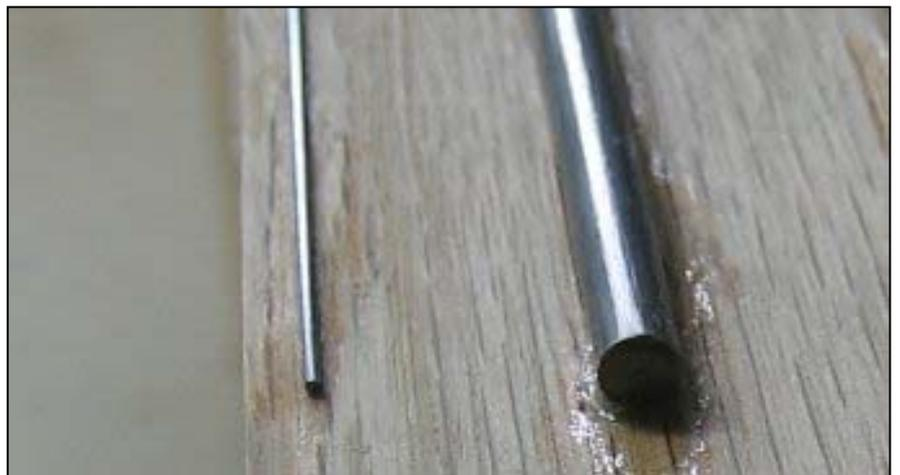
of the TE, and a smaller one to define the minimum thickness. The larger jig has two sets of wires for different size TEs. The wires are glued – I use cyano, but name your own poison – to a straight hardwood board. The two wires are spaced from each other (Fig 2) by an amount equal to the width of the rectangular stock you are going to use to make the TE. This may be the same as the TE width, or if not, the TE can be trimmed to the desired width later.
