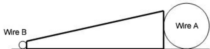
A little imagination will let you use existing jigs for other sizes of TE. For example, make a piece of 1/2 x 1/8 and then run it through your balsa stripper to bring it down to 3/8 x 3/32. Or slip a piece of 1/64 ply under the "fat" edge of the rectangular stock to produce a 1/2 x 0.1" TE. You get the idea. Enjoy!
