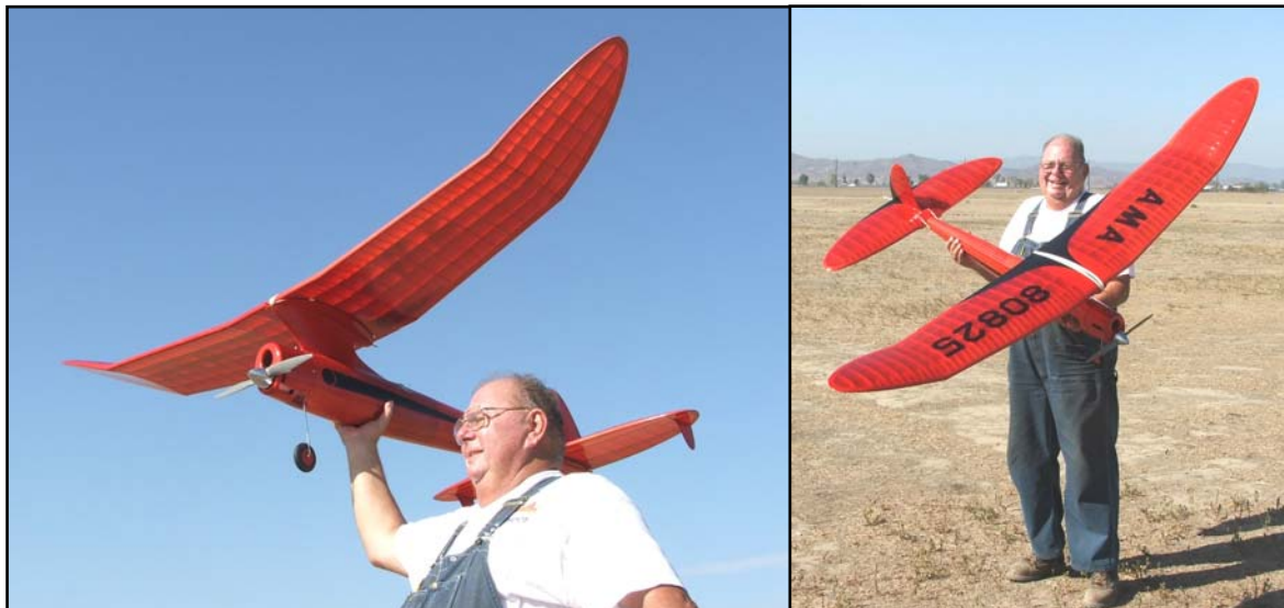
Gary Sherman's Sailplane shot with Kandy Koncentrate Red with black Aerodyne black nitrate trim and Black Domestic Tissue AMA numbers under Kandy Red
