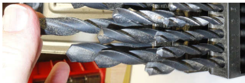
Figure 2 I select a drill about the same diameter as the tx is wide.
