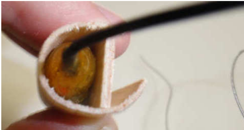
Figure 5 Hold the tube segment against the base with the tx in place. When everything looks and feels right, remove the tx and and CA the two together. The excess tube material can then be trimmed.
