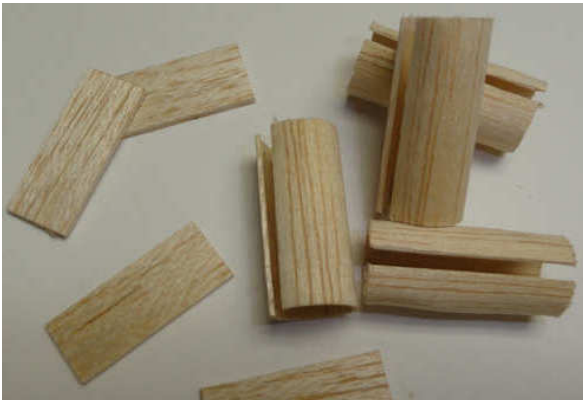
Figure 4 The 1/32 balsa tube is cut to length. The rectangles are 1/16 and will serve as the base of the housing.
