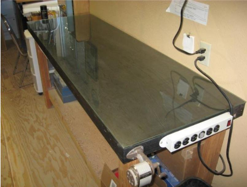
Before I start a model, I have the plans copied. After which, I cut the plans into reasonable sized pieces that can be attached to my 24" x 72" glass topped building bench. I spray the back of the plan with 3M type 75 adhesive which has about the same tackiness as Post-It notes.
