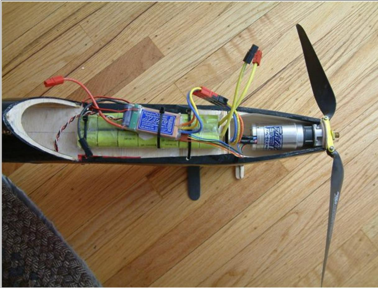
***This power unit; Aveox 1412/2Y with the Robbe 3.7:1 planetary gearbox, a 17x11 Aeronaut prop, an Aveox ESC and Battery of 14 Sanyo CP1300 cells is going in my new 108 inch 1150 sq inch Stardust Special.***
