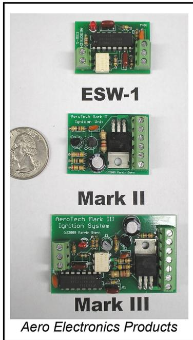
Replacing it are two new products. The first is the all new Mark II Ignition Unit. This is a standalone unit and does not include the ESW-1. The major feature is the protection afforded the output transistor and ignition coil in the event the engine stops prematurely with the points closed. If this happens, the unit shuts down immediately protecting the unit from possible overload and the ignition coil from burning up. It measures approx. 1-1/8 x 1-1/2 inches.
