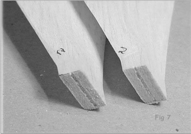
Fig. 7 Blades ready for insertion of new hub
