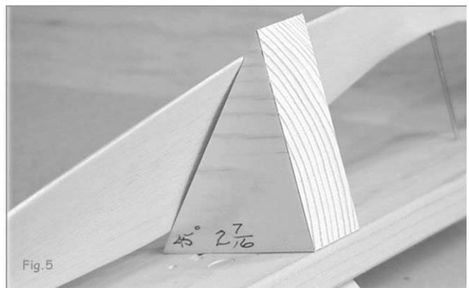
Fig. 5 Blade alignment jig to use with the Fixture of Fig. 4
