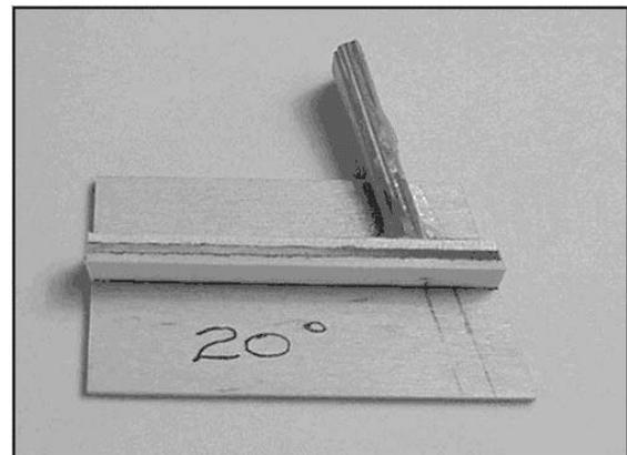
Fig. 2 Top view of the 20 deg. compound angle jig
