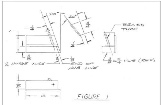
Fig. 1 Sketch of the jig used to drill the hinge angles
