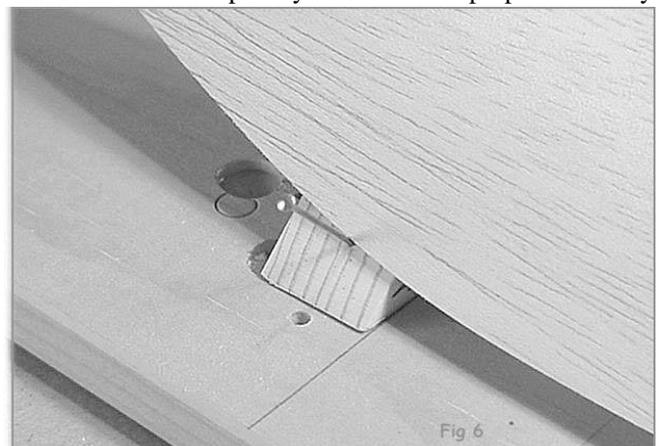
Fig. 6 Blade should clear the fixture base by about 1/4" (6 mm).
