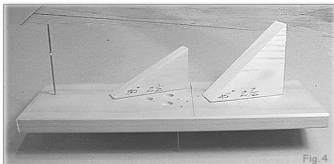
Fig. 4 Fixture for drilling hinge angles and setting proper pitch
