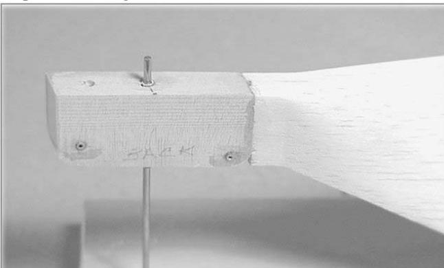
Fig. 8 Blade has been temporarily glued to hub for alignment in the fixture.
