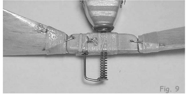
Fig. 9 Completed hub and blades of the folding propeller. Note look on hub for small rubber band to close low blade when folded.
