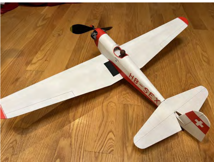
The control surface hinge lines are inked in.
