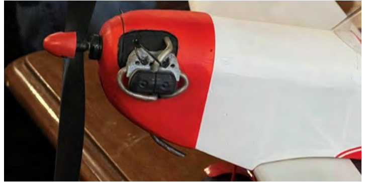
The scale VW engine is 3D printed.
