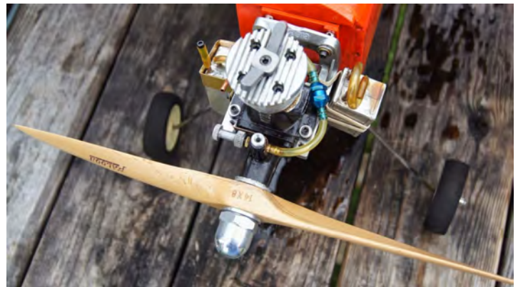
Drone for Texaco with intake restrictor and Falcon 14x8 prop. 810 sq. in. Holman Airborn short kit.
