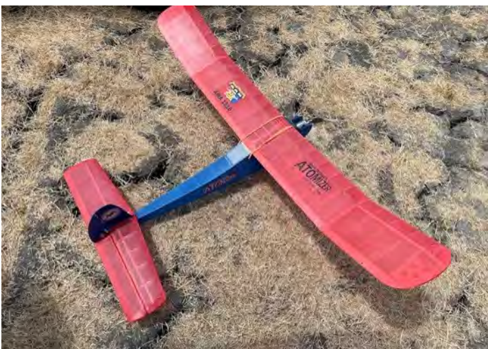
Mike's Atomizer. He flew it without elevator control. The nut holding the ball link to the elevator came loose during flight!
