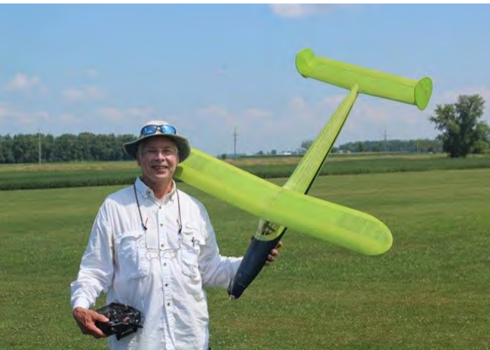
A 125% Smoothie for electroRubber class. Motor is Hacker A10-15S. Look at that green grass field!
