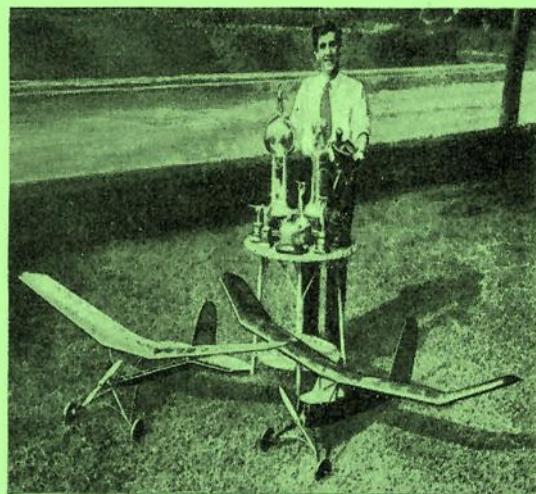
The low thrust line of the model on the right gave it a tendency towards spiral instability. Bassett countered this with generous tip dihedral and careful trimming.
