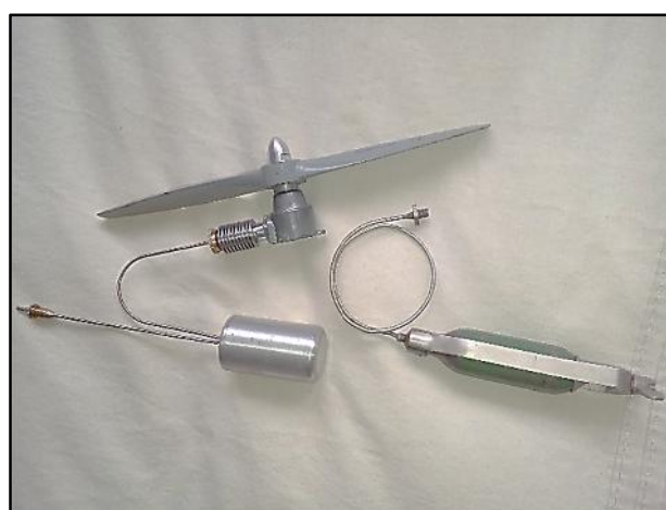
Gerard Moore's KK CO 2 motor plumbed to a Gasparin tank.
