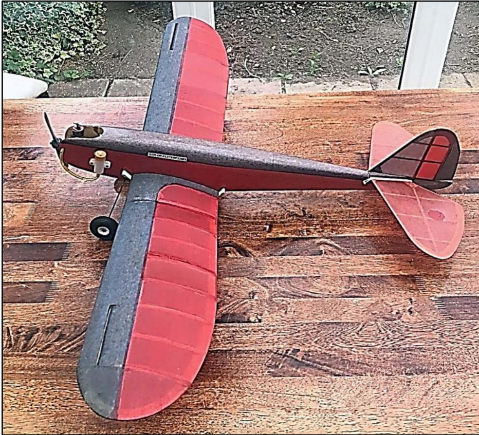
Miss Charlotte, designed by Andy Brough. Plans and article available on Outerzone. Note wing slots. Photo shows the original fuel tank arrangement, which was probably asking too much of the Merlin. Really needs a cockpit with a screen (as originally designed) or canopy as a finishing touch.
