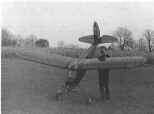
No modelers aren't getting smaller....even old timers have their BIG is BEAUTIFUL nuts. 14 ft. Quaker flash weighs 26 lbs., powered by 1.35 hp chain saw engine. Builder is Don Wolfer, Niles, Michigan.
