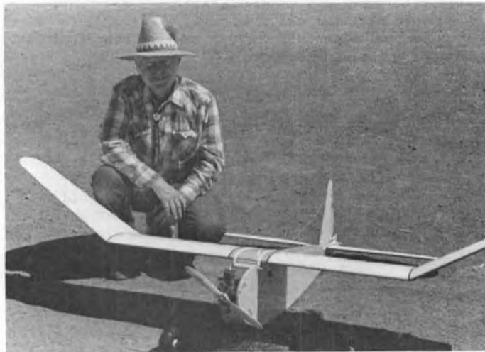
Jerry Doyle shows off his Super Cyclone powered Ehling R/C, ship sports a Flying Stab.
