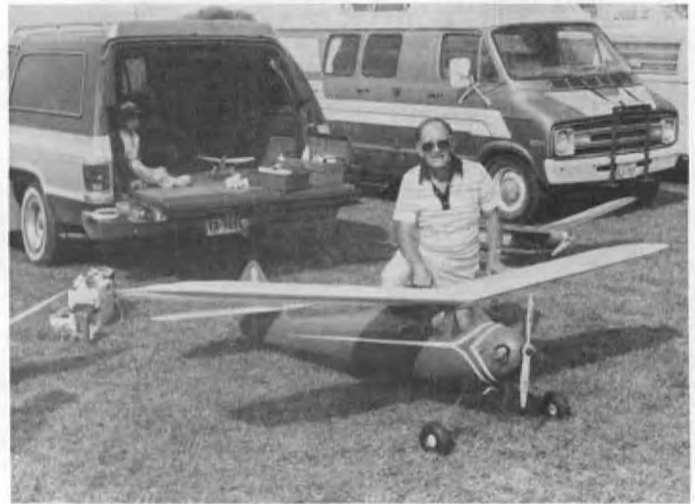
10 ft. span Shereshaw "Eaglet" built and flown by Marion Knight, Houston TX. Power is O.S. 'Gemini' 4 cycle twin.
