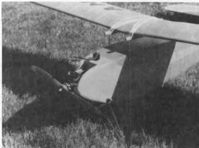
Very neat super cyke installation in Fred Lehmborg's PB-2. The coil location is very innovative, Fred is from Port Hueneme, California.
