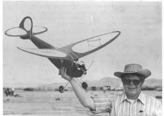
The Topper built and flown by Bill Booth who hails from northern California. This ship powered by a front rotor Ohlsson 23 was designed by Scotty Murray of the Old Brooklyn Skyscrapers Club.
