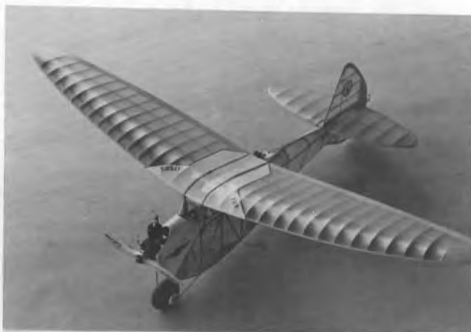
A beautiful Tambe, this one built with the airfoil shown on the M.A.N. plans. Powered by a converted Forster 29 Glo. The builder is Tom Heiser of Goodyear Arizona.
