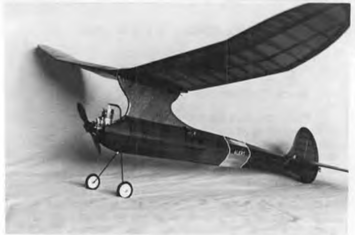
A lovely "alert" design by Michael La Torre. Ship was built by Tom Heiser. Power is a "77" products O.S. 25 conversion.
