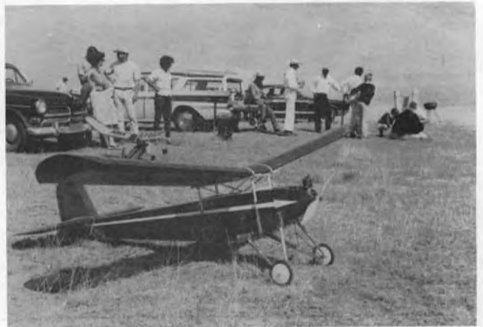
Ye Olde Editors K.G.3 at 1967 Denver Champs, Forster 99 powered heavy weight at 7 lbs. plus. An exact replica of Kovel-Grant original.
