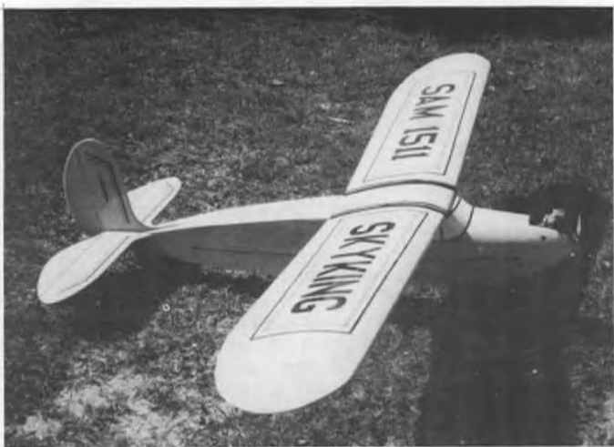
A big Peerless Panther, 82" span powered by a Glow .29. This is a very nice design.
