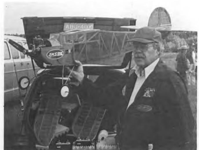
Steve Boucher with his OS 60 four stroke, equipped with Magneto for Texaco operation.
