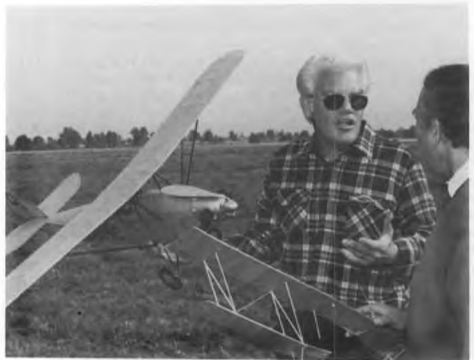
Mike Mulligan explains the action of his free-floating rudder to Fernando Ramos (Model Builder columnist). The gimmick rudder solved the spiral dive problems on his jumbo rubber scale. (Photo J. Adams)
