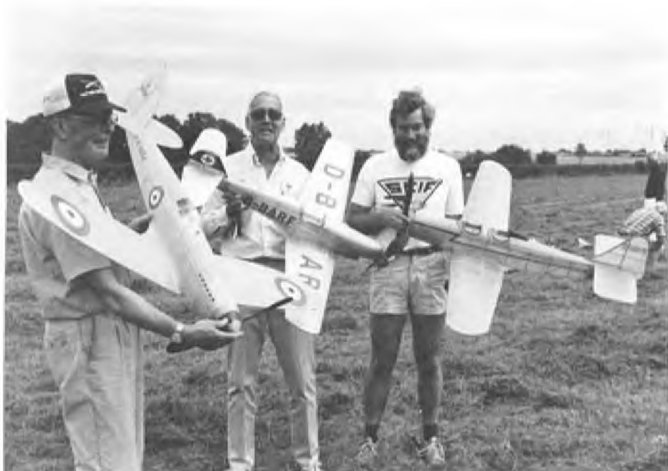
Mike Farrell shows off his "Bowden Midget" at Old Warden meet. Ship is powered by E.D. "Baby" diesel engine. Note the full span slats.
