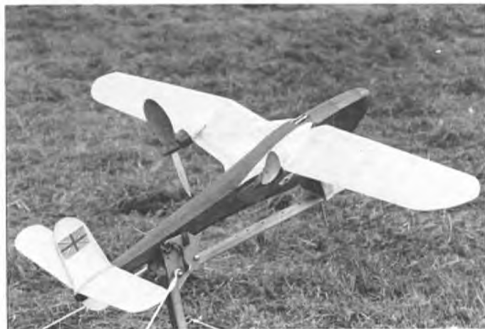
Shereshaw "Nimbus", R/C design flown by Jim Schelly. Power is a magneto equipped "Laser" engine.
