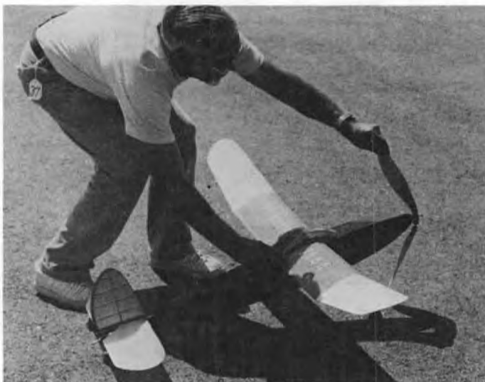
A "Lanzo Cabin". Remember the one with pop-up cabin dethermalizer? Well, this one uses a pop-up stab. This ship was being flown at Chicopee by Bob Moulton, Orland Park, Illinois. Photo: Harold Johnson
