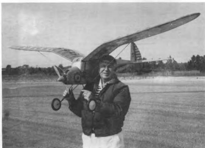
96" span "Modelcraft Spook" held by Cy Sapsford, our intrepid SAM modeler. This ship is powered by an old .51 O.S. and weighs 6.2 lbs. Cy says it's an excellent flyer.
