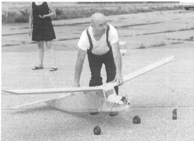
Ehling 8' gas model powered by an Atwood Champion. The modeler is George Murphy, Schenectady, NY.
