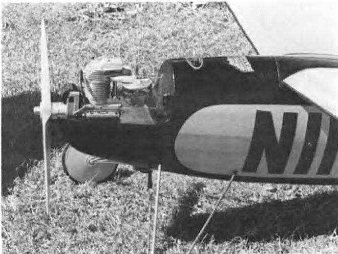
Close up shot of Laser engine equipped with a minimag. Flown at Old Warden by Jim Shelly in a Shereshaw Nimbus."
