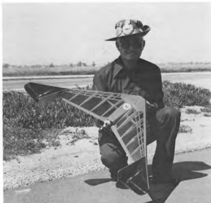
Very successful tailless design by Tex Rickard from 1938 Frank Zaic year book. This ship is powered by Cox .049 and flown in 1/2A Texaco.
