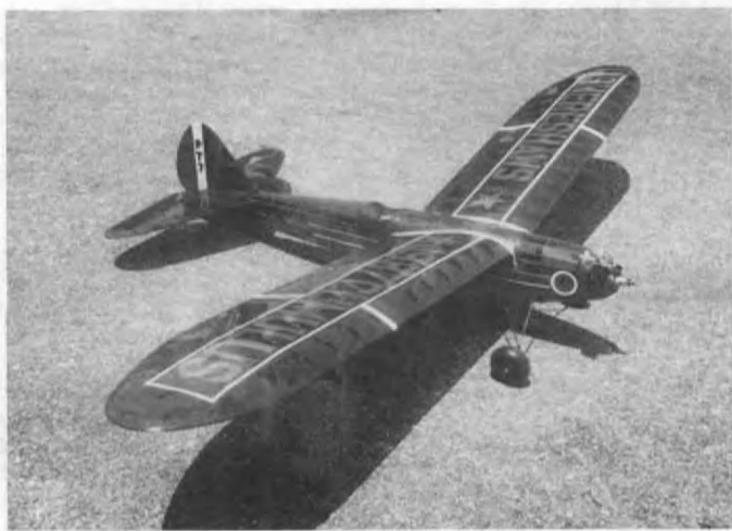
Lanzo's RC-1. Cy says this one's a great floater, powered by a .30 2-cycle (plenty of power).
