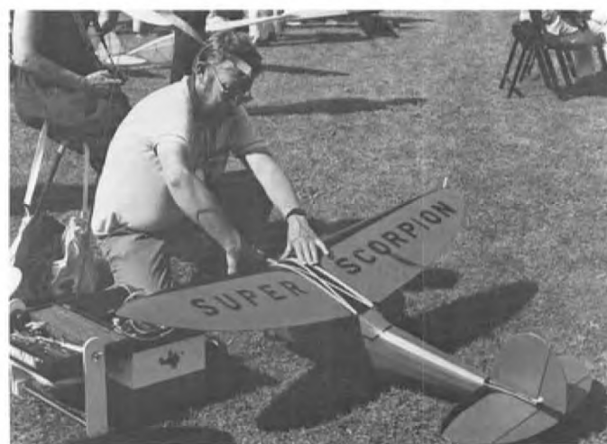
The Super Scorpion is a descendant of Scotty Murray's "Answer." This one, kitted in England, uses a Goldberg G-5 Airfoil. Very nice R/C ship.
