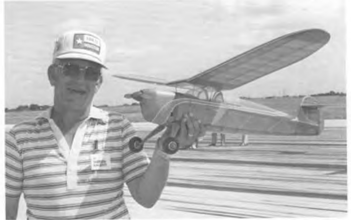
Marion Knight, Houston, Texas, holds his "American Eagle" for Class 'A' R/C. The design by Konefes was kitted by Comet and can be flown as mid-wing or low-wing. Original size was 45" span.
