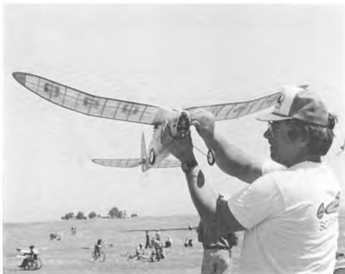
Al Heinrich, SCAMPS member from Costa Mesa, CA, tunes up his Ohlsson 23 powered "Cleveland Cloudster" at the Madera, CA, CHAMPS.
