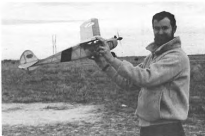
Steve Roselle, from the San Francisco Bay area, SAM 21, with his Bay Ridge Mike 1/2A Texaco. He uses a rev-up 8-5 prop. When the picture was taken, Steve was doing a "miles per gallon" check -- he uses K&B 1000 fuel and gets about six minutes.
