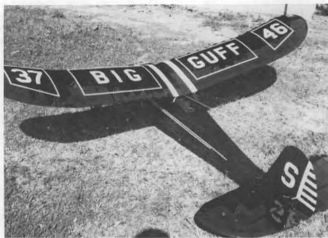
A very rare VB-2 designed by Vartanian and Bellatonic. This ones a winner powered by .90 4-cycle.
