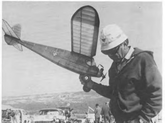
Larry Clark, one of the S.C.I.F.'s from North Los Angeles, holds his "Westwind" big brother to "Miss Tiny". The ship is powered by an Ohlsson 23. The ship was kitted by Modelcraft and was a Barney Snyder design.
