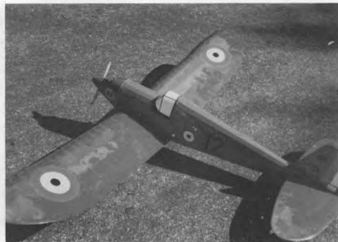
A "Sky King," designer unknown. This one powered by a Saito .45 4-cycle is 88" span (looks like a Fairchild 24 in its ancestry).
