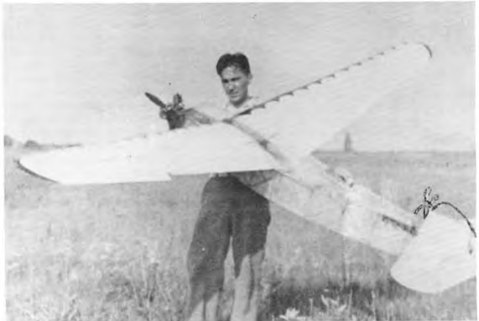
Elmer Wasman holds his 10lb R/C model which won 3rd place in 1937. It has rudder/aileron and elevator control, also engine cutoff. Rearview of Wasman's plane shows the air-driven, 4-bladed propeller, mounted on front of the fin for power for moving the control surfaces.
