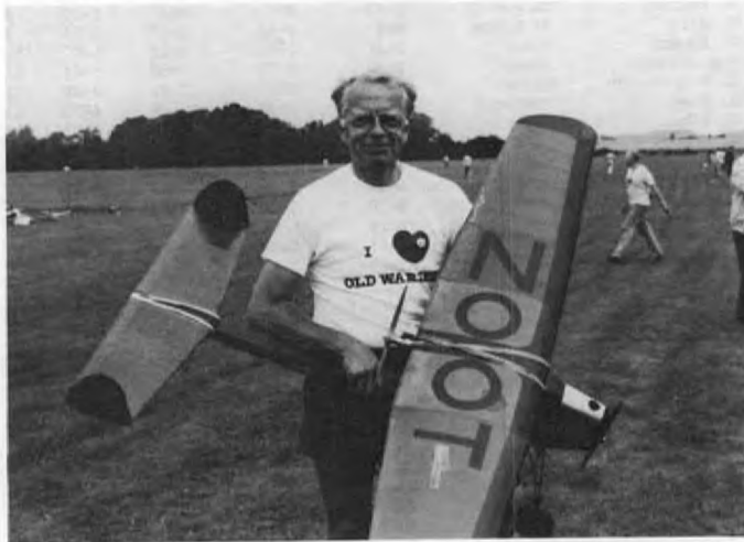
SAM 35 Spark Plug, David Baker, and his Push-Pull H.A. Thomas & J. Sadler design. Ship is powered by twin P.A.W. Diesels.
