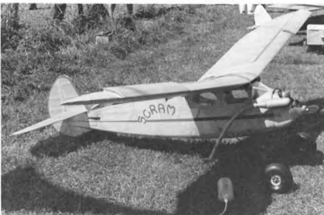
Gorgeous R/C "Scram," by Jeff Smith, of Rugby, Midlands. Ship is powered by Webra 61 with diesel head. How about those wing slots?
