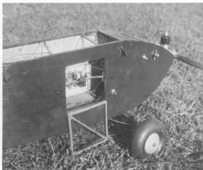
Guff side view showing receiver suspended on rubber bands. The Guff had an 8 ft span and weighed 8.5 lbs.
