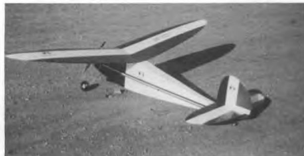
A competitive "Super Clipper" for sale, 10 ft span with a throttled Forster 99 for power. Micafilm cover, 8 pounds
