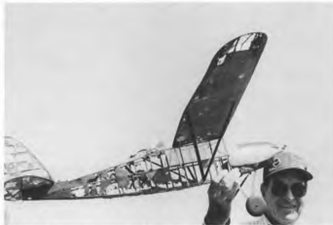
Chet's famous 45 year old "Puss Moth", now in the AMA museum. You can see the undercambered airfoil in this picture.
