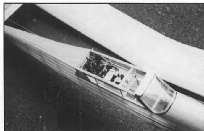
The R/C installation in this unique 300 sq.in. rubber model (the ultimate DT!). The Cannon Rx/servo block and 100 Mah battery weighs just under 3 oz., total wt. is 16 oz. After trim and balance adjustments, the model made 2 flights over 12 minutes!
