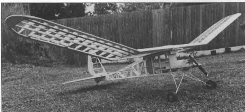
The "Colossus", 9 foot span Aussie model by John Wallen of SAM 84, Queensland.. From an 1947 Air Trails plan. Powered by Salto 65 4 stroke
