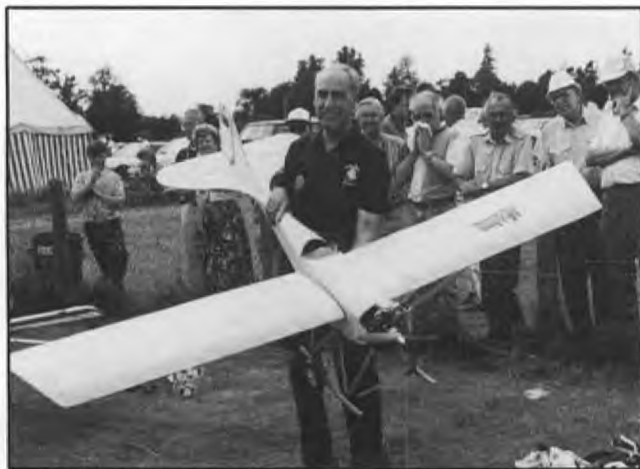
Arthur Fox's Twining O1-P1 at Old Warden. Each rib built up, covered with Solartex, powered by 90 four stroke
