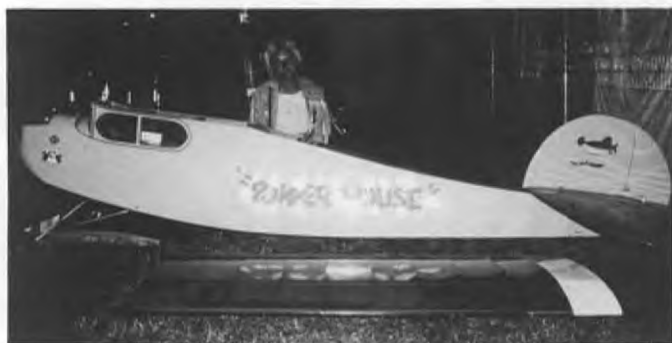
Cohen's monster 14 ft. "Powerhouse", Quadra power, has 4,365 sq.in. wing. Momocote covered and an extra 2 1/2 gal. fuel tank.
