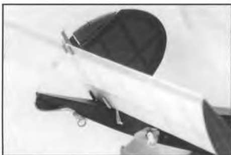
Reid DT detail. Note fuse location and trip line tube below elevator keys.
