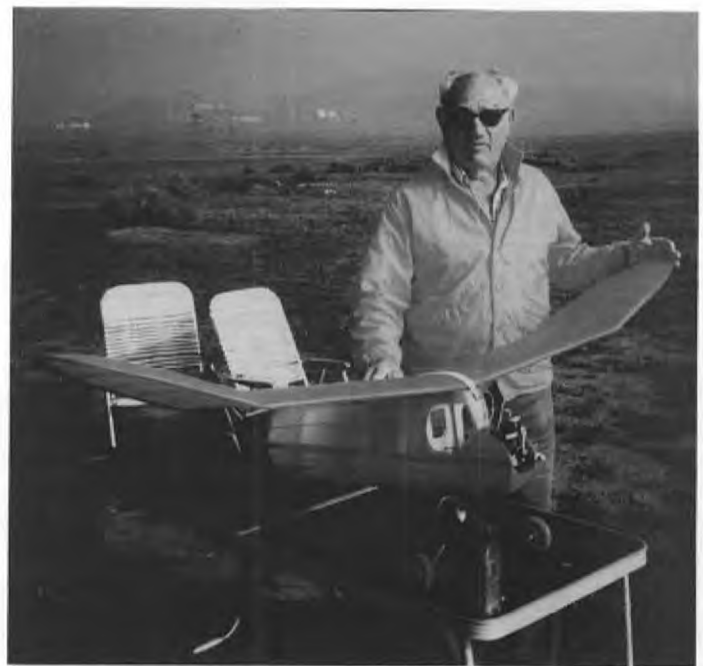
Sal Taibi with his newly approved 6 ft. size Brooklyn Dodger. Red, white, and blue colors. The Orwick 64 power is turning a 14-6 prop. Plans and kits available, see page 18.
