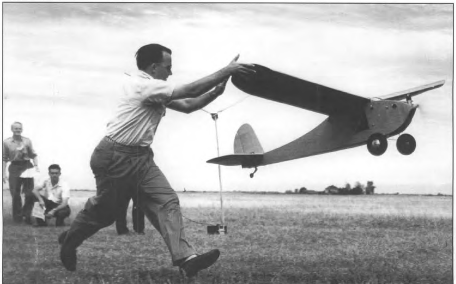
Walt Good launching the RC Guff with Bill at the controls - only Bill's feet are visible. The Long twins are at the far left with their judging sheets. The Guff had rudder only and engine cut-off. The engine was an Ohlsson 60. The RC gear was a single channel Beacon Rx and Tx with a 4 spoke escapement.
