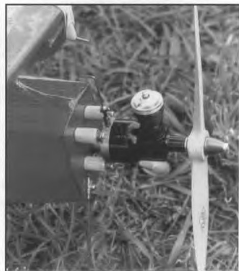
John Schneider's controversial mount for a Cox .049. Makes for easy starting by being able to choke those cranky 1/2 A engines
