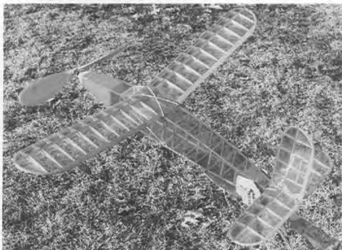
A dyed mylar covered "1 1/2" built and flown by Les De Witt. This unusual de la Mater design adapts well to this unusual covering material, retains it new appearance for years. B&W picture does not do beauty of this covering justice. It is gorgeous! And outlasts tissue.
