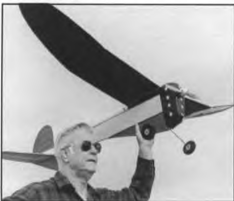
Russ Schuppner's fine "Record Hound", Astro cobalt .15, 14 cells
