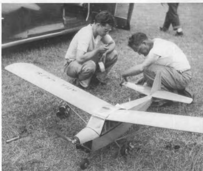
Jim Walker adjusts tail of his proportional rudder & elevator, variable speed engine and trike gear.
