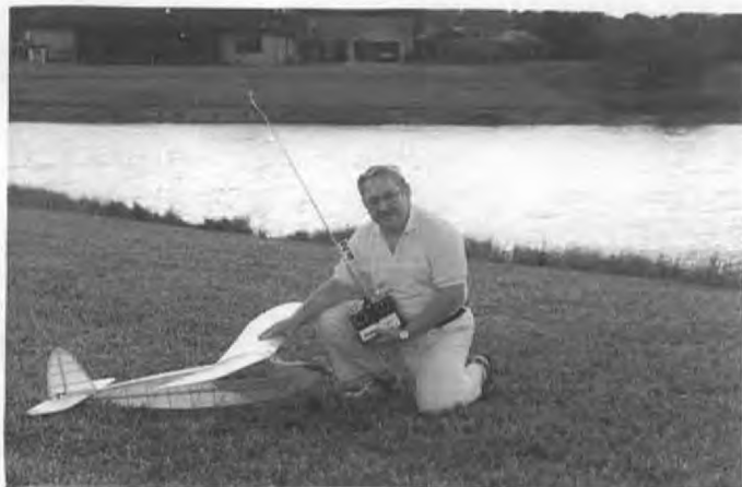
Norm Rosenstock with his 600 sq.in. MISS AMERICA powered by a .15 diesel. Weight is 34 ozs. All silk covered with epoxy paint trim Two channels (elevator & rudder). Fuel tank 14cc. Longest flight 28 minutes.
