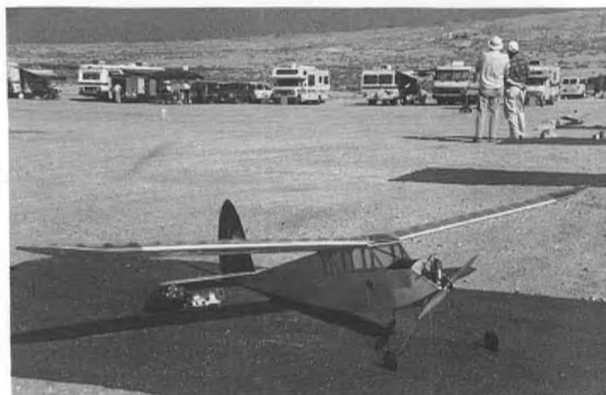
A 1936 "Flying Quaker", powered with our old favorite, the Brown "D". The wing is covered with Monocote with a Micafilm "skin" on the fuselage. This "bird" was built by George Tallent of Picacho, AZ. Reich photo
