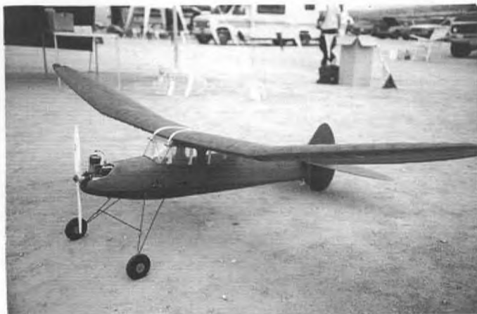
A beautiful "Blue Flamingo" R/C by Walt Geary of Atlantic City, NJ. Power is O&R 60. The model is covered with Sig Silkspan.
