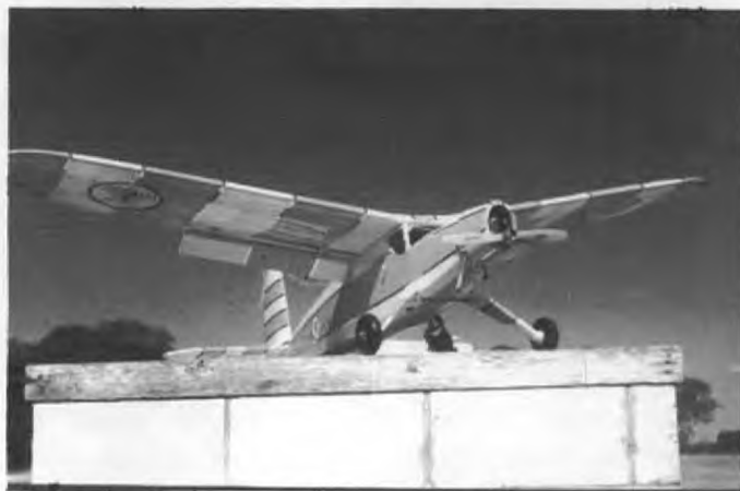
From Bendigo, Australia comes this photo of M.L. Matheson's 80% "Sky King". This "bird" is from the Feb. 1937 issue of Air Trails. Span is 72", with Enya 40.4cc and weighs in at 5-1/4 lbs. Uses a Futaba radio with the 4th servo used for flaps to 30°, using 4 rods and bellcranks. Requires full down to compensate for nose-up couple on landing.
