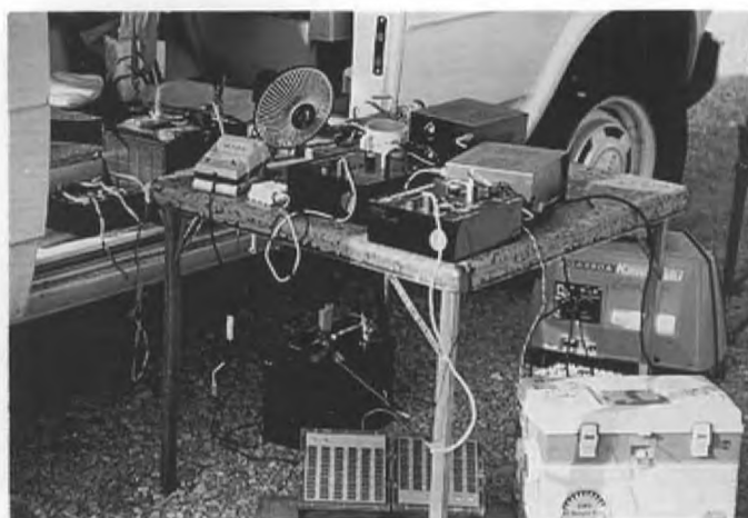
Jerry Smartt from Warsaw, MD is a true electric aficionado! Let's see...the generator supplies power to the inverter, which in turn supplies 12V to the chargers, which are backed up with 12V auto batteries on and under the table which are recharged by a small solar panel! The 12V fan cools the entire mess!
