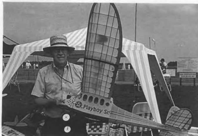
Howard Robinson from Shelby, OH displays his O&R .60 powered "Playboy Sr. Cabin" all wrapped up in a flat-finished red silk fuselage.
