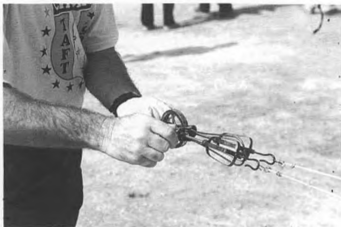
Vic Cunningham's special twin canard pusher winder, a modified egg-beater that winds 'em both at once!
