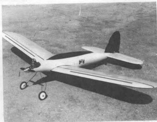
COL. BOWDEN'S PLN-4 DESIGN (1936) BUILT BY ROSS THOMAS, SANTA ANA, CA. POWER IS A BERNHARDT CONVERTED MERC0.
