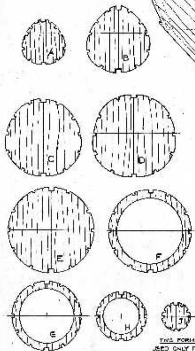
FUSelage FORMERS 1/16" THICK 1/16" DIA. EACH REQUIRED
