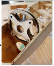
And below are the body formers on the mandrill in a more advanced stage
