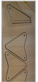
Was able to cut some nice control horns complete with 1.5mm hole for clevis.
