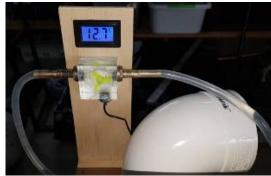
Some sort of alternate **Fume Extraction** system is needed because the one provided, was not, in my estimation powerful enough, I used an old Dyson Vacuum cleaner and a viable motor controller, 90mm storm water fittings, together with 90mm flexible domestic ducting and placed close the exit point to outside.
