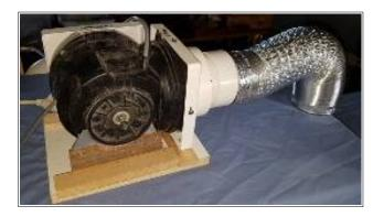
Addition of an **Air Assist** nozzle (read air blast to reduce the burn marks), which I 3d printed from <a href="www.thingiverse.com">www.thingiverse.com</a>, and some sort of compressor to supply the air at a very low pressure.
