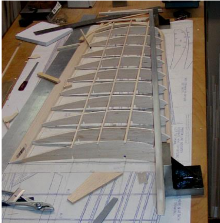
This shows all three top spars installed on the left wing tip panel. Notice how straight they are. :O)
