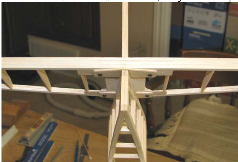
This final picture shows the removable fin and stab mounted to the fuselage via the stab platform.
