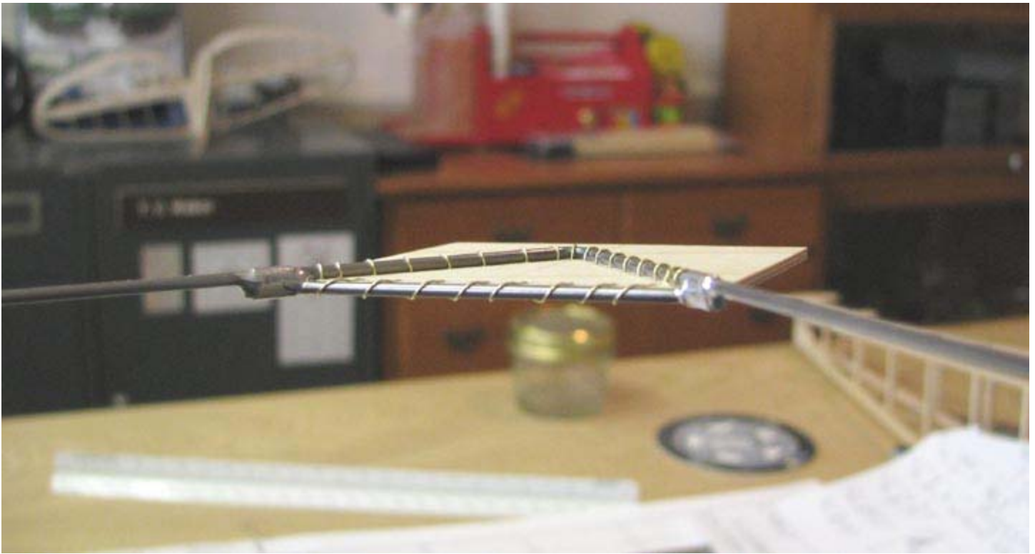
This shows a trial fit of the landing gear's plywood plate in the fuselage structure.....Tandy
