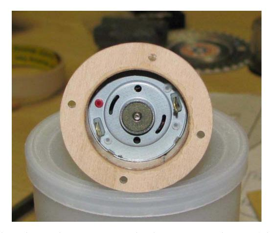
This picture shows the Speed 400 motor mounted in the motor tube with spinner/adapter attached and the assembly laid on the plans to check the location of the rear face of the spinner. Notice that the top of the rear mounting ring has to be trimmed down later to fit inside of the cowl contour and the fourth support gusset added at the top.......Tandy.
