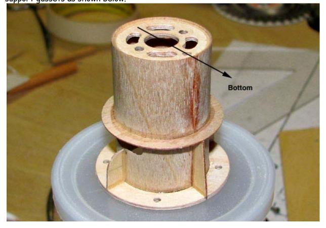
This is a close up view of the rear mounting ring from the back of the mount.
