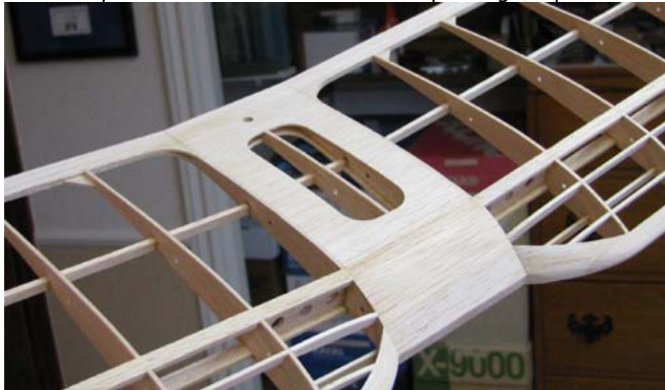
This is just a shot of the complete wing showing the planked center section.
