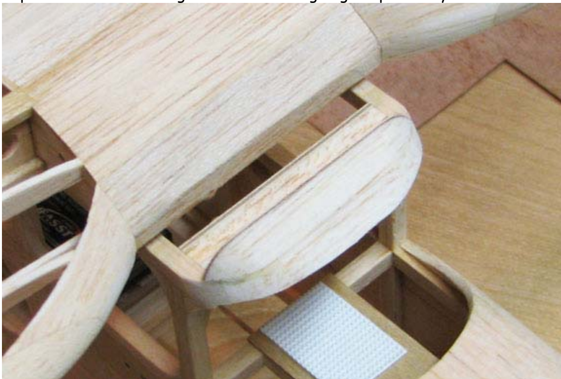
This picture shows the wing's notched leading edge in proximity of the cabin stop.
