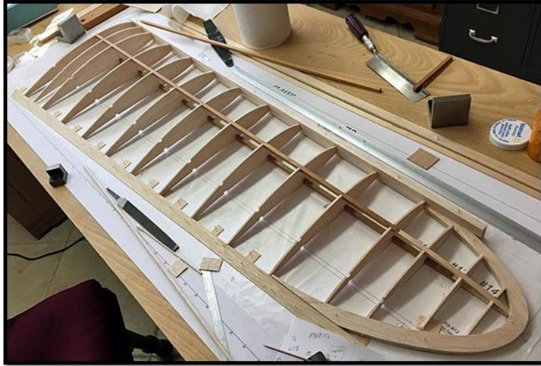
This view from the wing root shows the top main spar installed on the right wing panel.....Tandy
