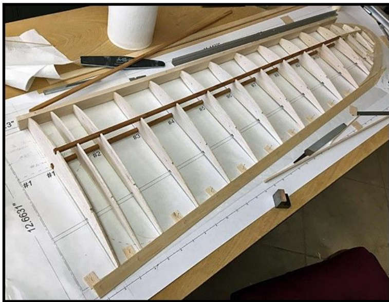
This view from the wing root shows the top main spar installed on the right wing panel.....Tandy
