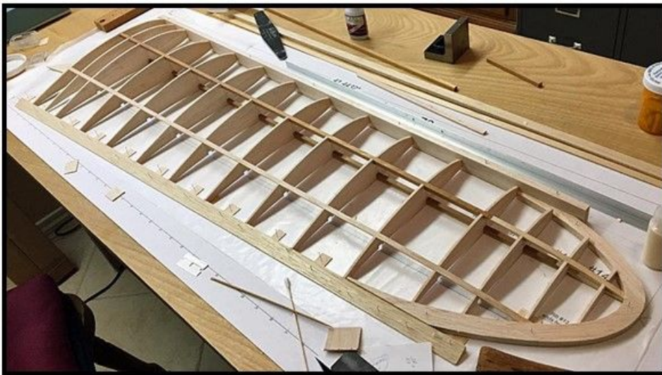
This view from the wing tip shows the top rear spar installed on the right wing panel.
