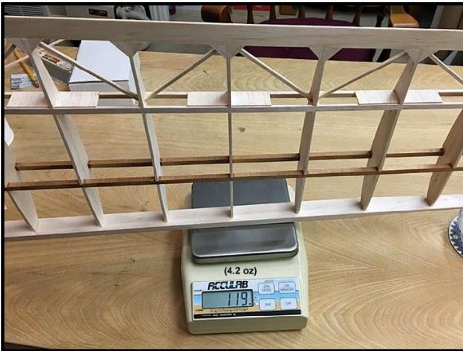
The weight of the right wing panel is 119 grams (4.2 oz) at this point.....Tandy
