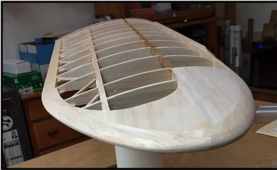
The weight of the right wing panel is 119 grams (4.2 oz) at this point.....Tandy
