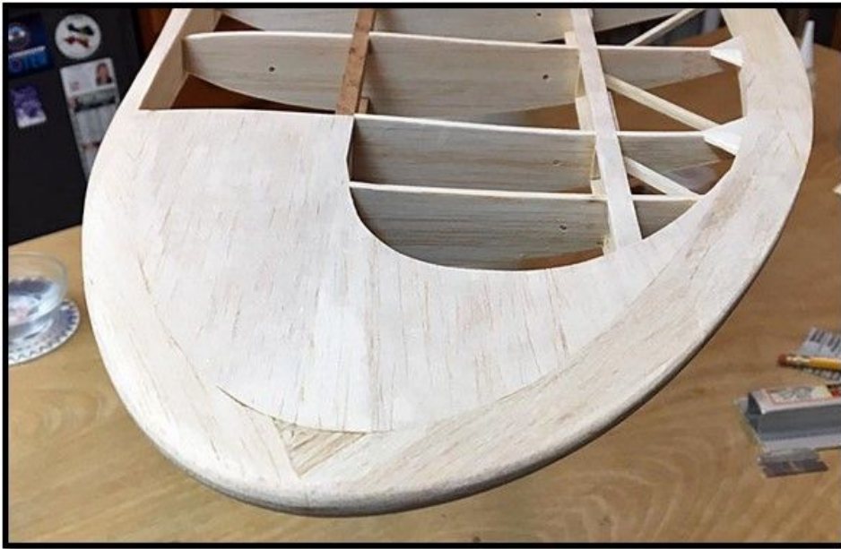
This tapered filler was pre-shaped for the bottom rear spar.
