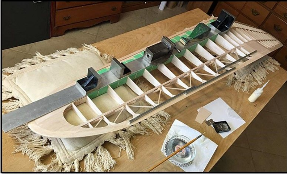
This picture shows the little balsa prop under the leading edge to stabilize the wing panel on the pillows. Also three 1/4" square steel rod were placed on the trailing edge of the panel as counterbalance to further help stabilize the panel on the pillows.
