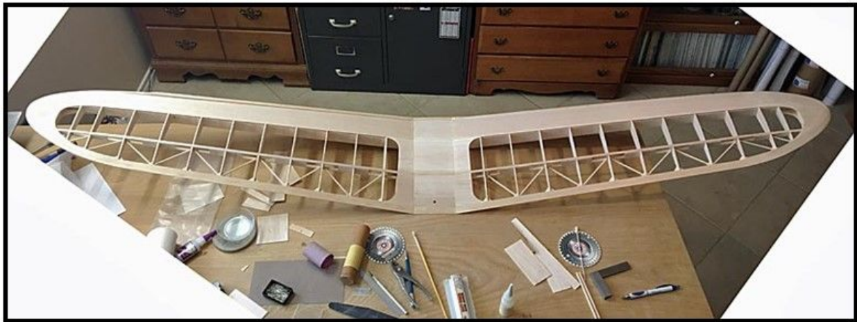
This picture of the wing was taken to show all of wing's top planking. The bottom of the center section's planking will be completed tomorrow.....Tandy
