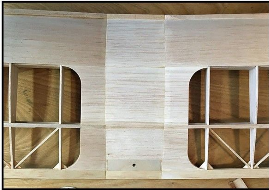
This picture of the wing was taken to show all of wing's top planking. The bottom of the center section's planking will be completed tomorrow.....Tandy
