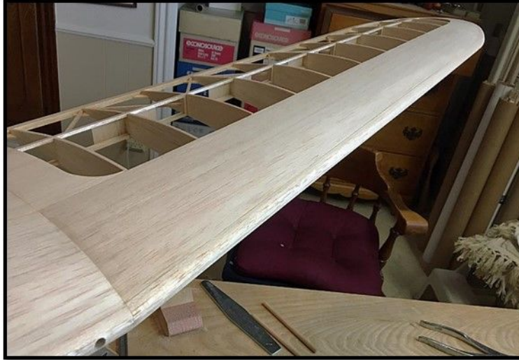
This is a close up showing the left wing panel's shaped leading edge.
