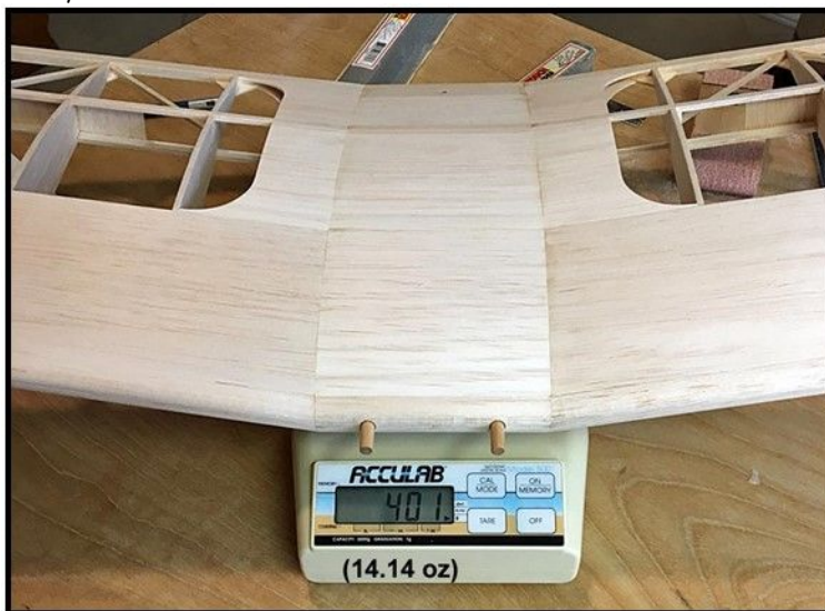
The uncovered wing structure weighed in at 401 grams or 14.14 ounces as shown below, which is 22% of the model's total 64 ounce weight.....Tandy
