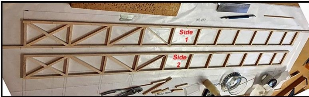
Finally the second side of the fuselage's primary structure was framed up as shown below and will be left to dry overnight.....Tandy
