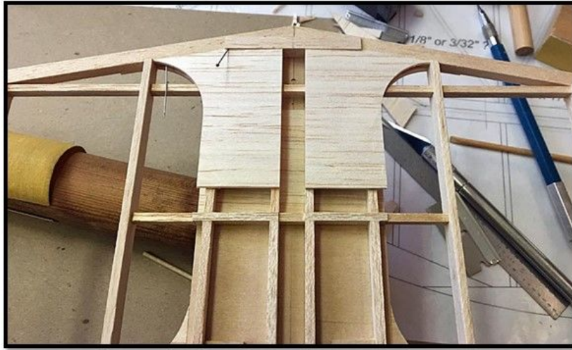
This picture shows the stab's top planking complete. Notice the well-defined 3/8" slot for the fin base.
