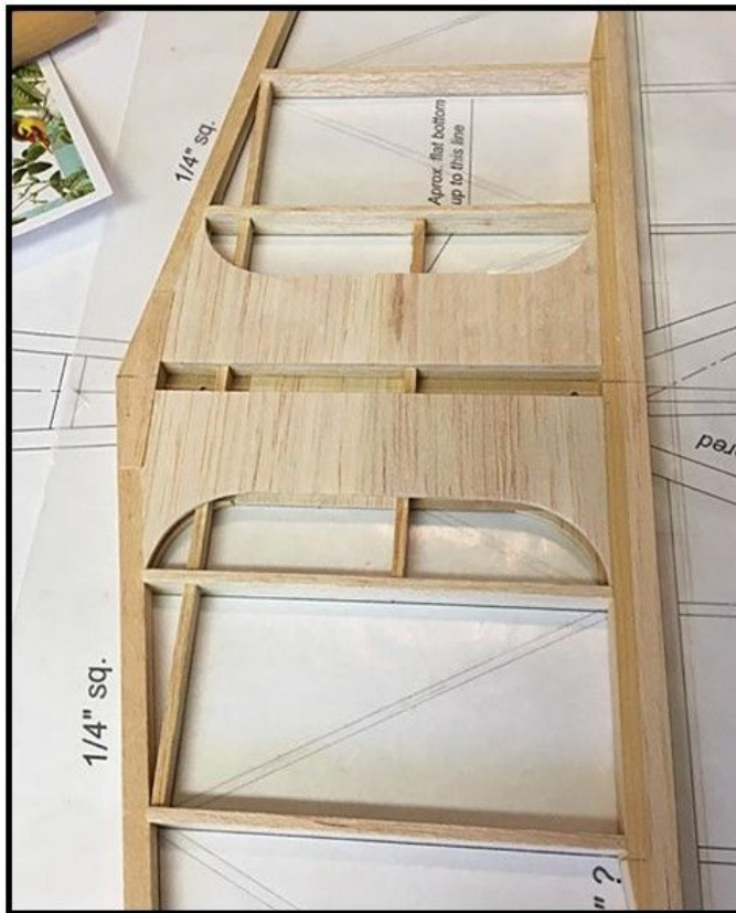
This picture shows the stab's top planking complete. Notice the well-defined 3/8" slot for the fin base.
