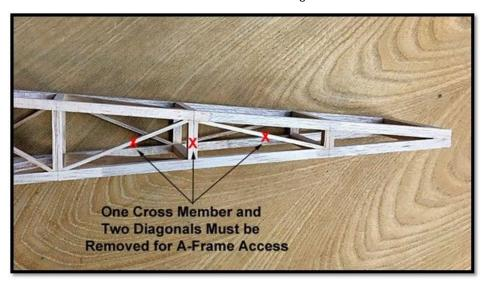
This shows the fuselage structure after the three members were removed.
